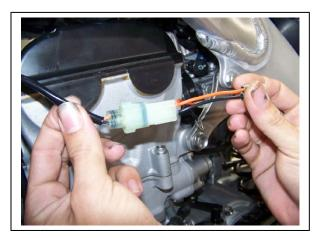
3. Route the harness up the left side of the frame through the factory wire guide, above the left radiator to the front of the steering neck.
