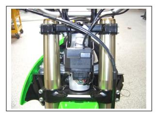
6. Next you can install your light to your forks and ensure that you have clearance between the back of the racelight and your ECU. Make sure the steering turns lock to lock and ensure adequate clearance in all positions.
